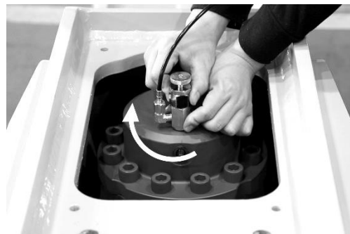
6. Connect adapter to inlet port.
