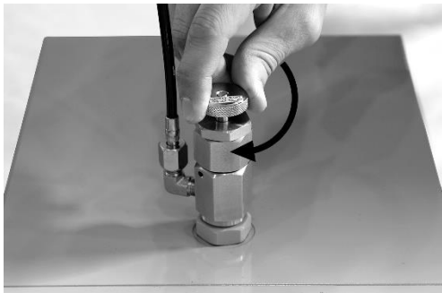
5. Tighten top section of adapter.
