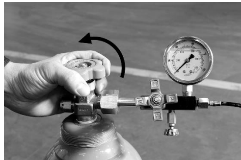
6. Open gas bottle valve SLOWLY. Quick valve opening may cause damage on the gauge.
