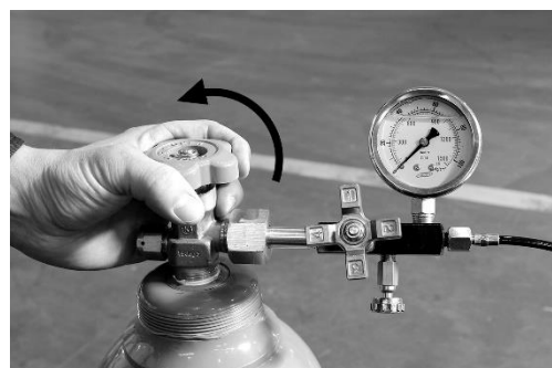
8. Open gas bottle valve SLOWLY. Quick valve opening may cause damage on the gauge.
