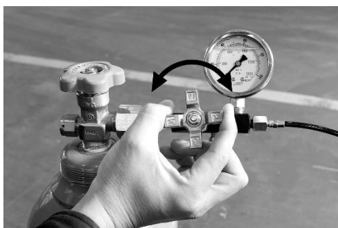
9. Open 3-way valve slowly, charge N2 gas up to 65 kg/cm 2 , close the valve.
