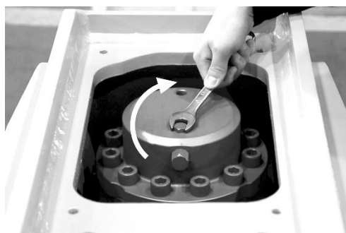
14. Assemble valve cap.
