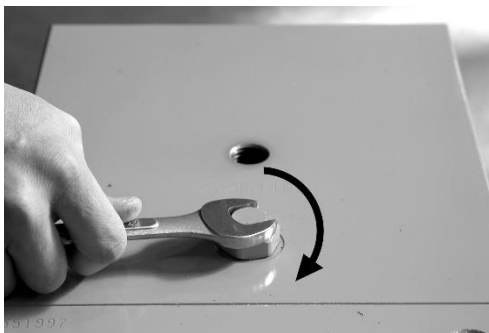
11. Assemble valve cap to the inlet port.
