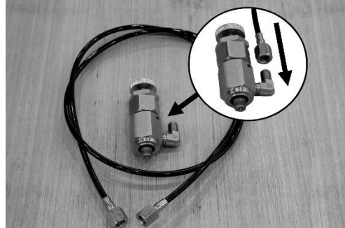
2. Connect hose to adapter.
