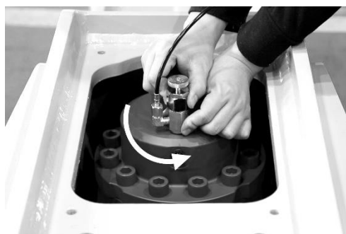
12. Remove gas charging adapter.
