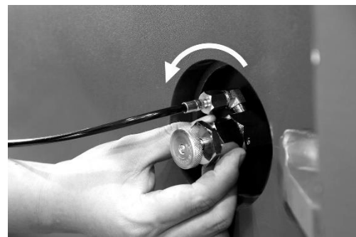
11. Disassemble adapter from the inlet port by loosening middle section of adapter.
