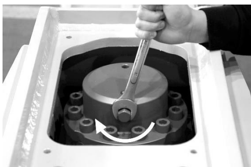
13. Assemble needle valve cap.
