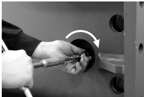
12. Assemble valve cap to the inlet port.
