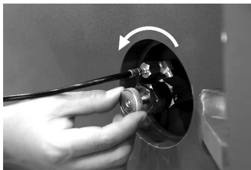
10. Close inlet port by loosening top section of adapter.
