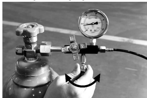
8. Drain the gas to 16~18 kg/cm 2 upon ambient temperature of job site.
