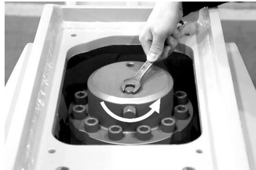
2. Remove valve cap.
