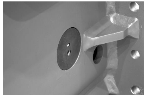
13. Assemble rubber plug.
