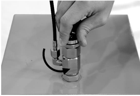
9. Close inlet port by loosening top section of adapter.
