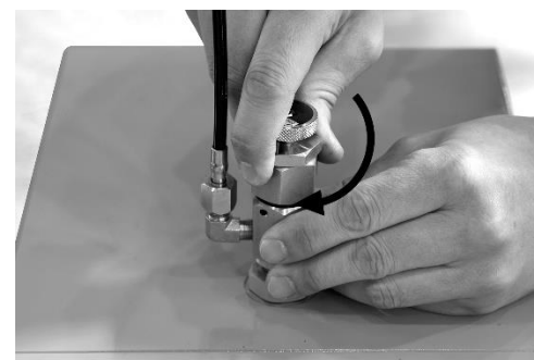
4. Fit adapter on the inlet port by tightening middle section of adapter.
