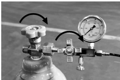
4. Close gas cylinder valve, connect gas charging kit to gas cylinder, close 3-way valve and drain cock.
