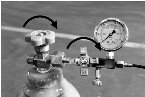
5. Close gas cylinder valve, connect gas charging kit to gas cylinder, close 3-way valve and drain cock.
