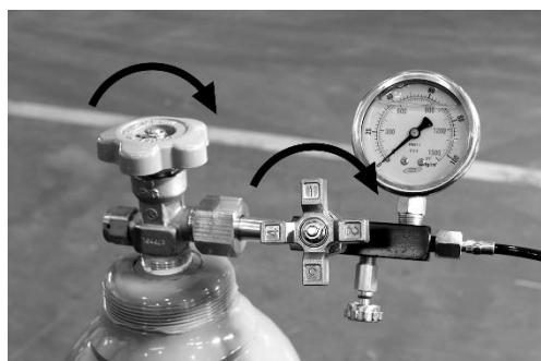
3. Close gas cylinder valve, connect gas charging kit to gas cylinder, close 3-way valve and drain cock.
