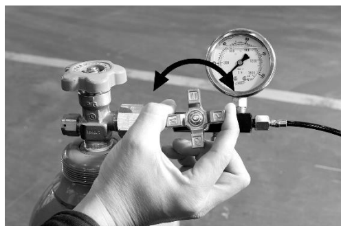
7. Open 3-way valve slowly, charge N2 gas up to 20 kg/cm 2 , close the valve.
