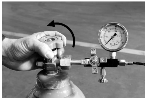
7. Open gas bottle valve SLOWLY. Quick valve opening may cause damage on the gauge.
