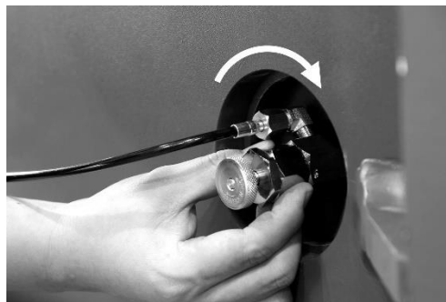
5. Fit adapter on the inlet port by tightening middle section of adapter.
